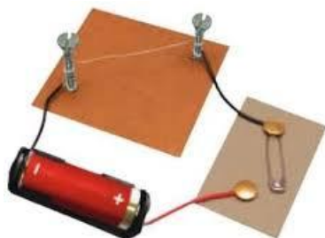
Fig. 4.5: Heating effect in a wire
